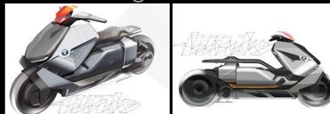
The BMW Motorrad Concept Link also deliberately showcases the technology used as part of the design package. That is why the side panels don't completely cover the side section at the rear. Instead they stretch across the vehicles side like little wings allowing views of the technical elements like drive unit, cooling ribs, single-sided swing arm, spring strut and tooth belt. At the same time they help improve aerodynamic air flow.
