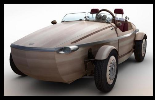
The goal of this material choice is to "be able to capture the developing relationship between people and their cars in the way it changes in appearance over the years." oyota designers picked a variety of types of wood for different parts of he car, including the exterior panels, frame, floor and seats. The design blends a two-seat, open wheel layout with a look influenced by the sport scar of the early 19th Century, while the wooden surfaces howcase a clear inspiration from the boat world.
