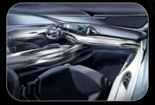
A logical and spacious center console divides the interior space through its length axis into two separate halves. Combined with the curved, floating screen, the Central Control Panel (CCP) creates a new user experience through a tactile and considered control lay-out.
