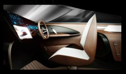
The user interface of the multimedia and entertainment system is installed in a 15€² touch screen on the dashboard, which the guests can also use. Owners have their own cluster with a dedicated display for monitoring engine status and navigation.
