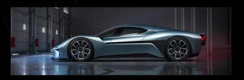
It will also do 0 to 200KPH (124MPH) in 7.1 seconds and 300KPH (186MPH) in 15.9 seconds. The EP9 can't, however, complete a quarter mile stretch in under 10 seconds (at 10.1 seconds, it's pretty close however.) The complete car weighs 1735KG, with 635KG devoted to batteries alone. Those power packs are interchangeable too, with a fresh set lasting 427 kilometers (265 miles).
