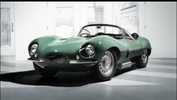
All nine will be new cars, but use period chassis numbers – presumably from the cars lost in the fire. The bodies will be hand-wheeled from magnesium alloy, and the cars will feature period Dunlop disc brakes, Dunlop tyres and two-piece riveted magnesium alloy wheels.
