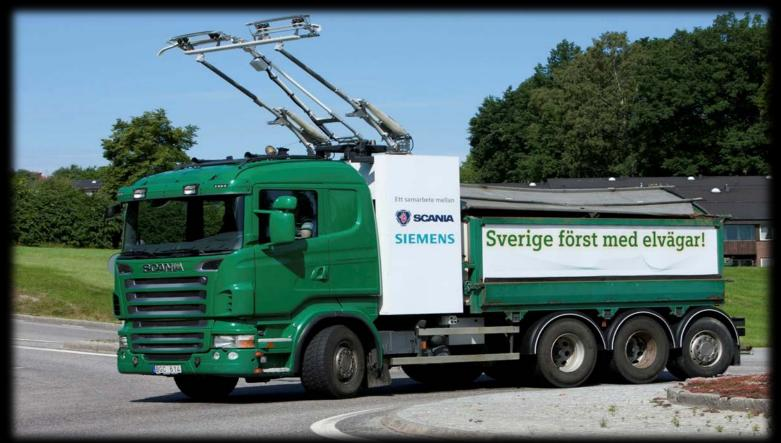
The buses and heavy cargo vehicles are powered by electricity from overhead cables
