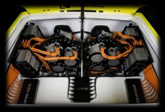
The twelve compact, liquidcooled permanent-magnet synchronous electric motors which are the signature piece of the SLS AMG Coupé Electric Drive: each electric motor delivers 138 kW and 250 Newton meters.
