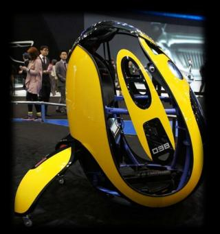
The scooter-like vehicle weighs 80kg (about 176 pounds) including the the battery and is just over three feet wide.
