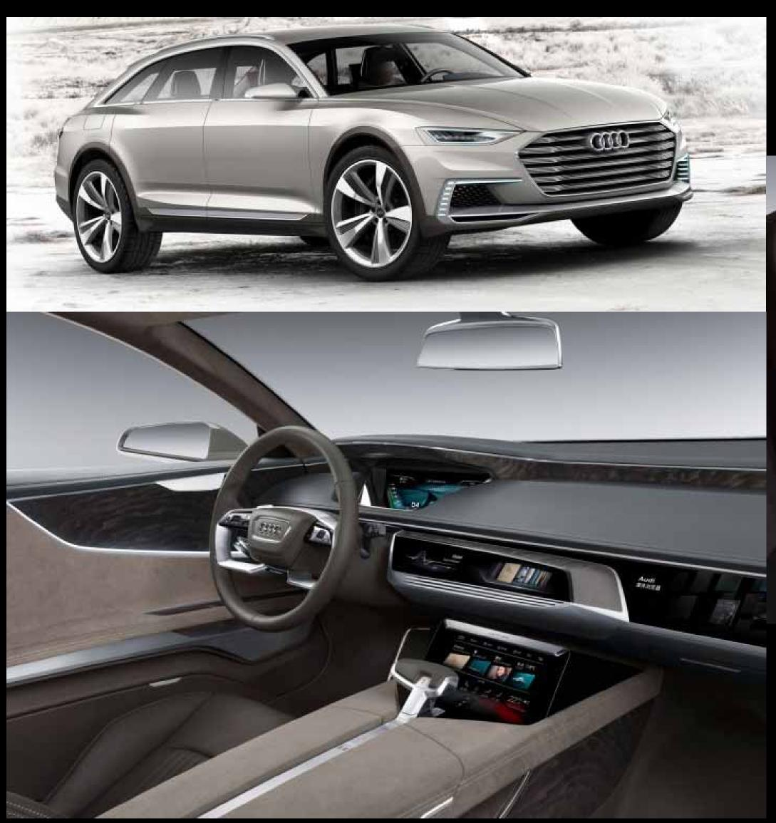
The concept is powered by a 540 kW / 734 hp plug-in hybrid system featuring a 4.0 TFSI engine – a V8 with twin turbochargers.
