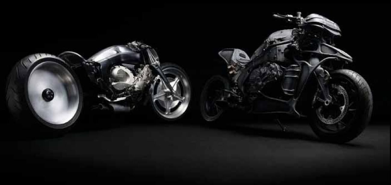
The illusion of a dramatically low seat height and narrow motorcycle is enhanced by the use of a 23-inch front wheel and a 20-inch rear wheel. More nicely manufactured details made from aluminum like covers for fuel tank and radiator or handlebars are completing Kenji Nagai's artificial craftsmanship.
