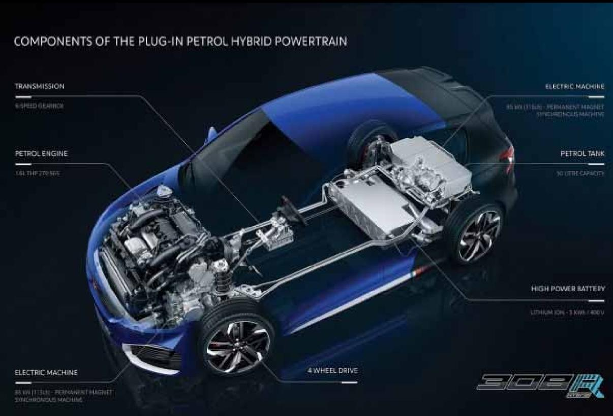
The color scheme combines a blue paint with fluorescent pigments and glass particles with a rear section finished in matte black – a livery similar to that introduced with the 308 R Concept. The plug-in powertrain combines three sources of power, each capable of moving the vehicle independently of the others.
