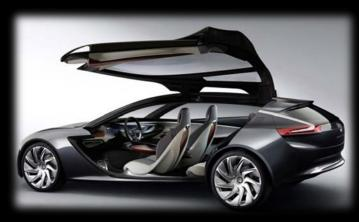
The large gullwing doors allow easy entry and egress for front and rear-seat passengers. The Monza Concept is a 4.69 meter long vehicle, with a very low stance (1.31 meters) and a shooting-brake rear section. The front end is characterized by a sculpted hood with the trademark center fold.
