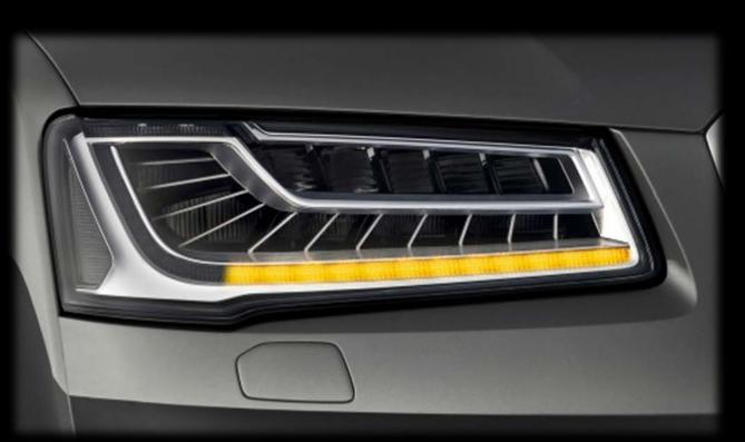
The Audi Matrix LED headlights mask the relevant sections of the high-beam by dimming or shutting off individual diodes. Very bright illumination is preserved in the remaining zones. The Audi Matrix LED headlights also feature navigation-based cornering lights and, in cooperation with the night vision assistant, a marker light that warns the driver of pedestrians in the dark and which also alerts the pedestrians.
