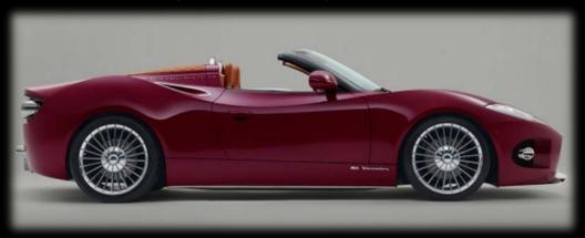
The Spyker B6 Venator Spyder features an allcarbon fiber body mounted on an allaluminum chassis, and is powered by a rearmid-mounted V6 engine delivering 375+ bhp. Power to the rear wheels is transmitted through a six speed automatic transmission.
