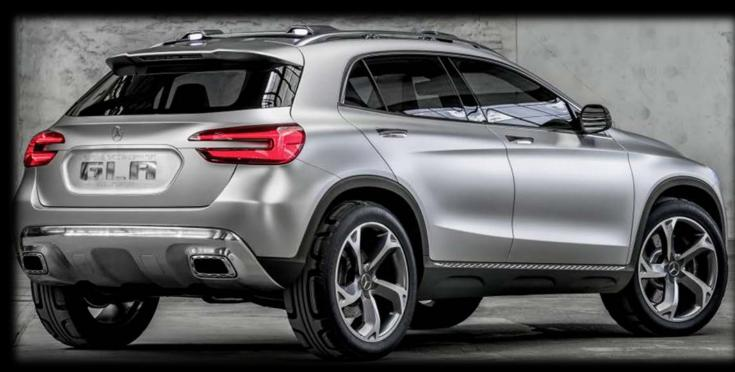
While the GLA is a touch larger than the A hatch, measuring 4.38 metres long and 1.57 metres tall, both models ride on the same 2.69 metre wheelbase. In concept form, the GLA is driven by the same 155kW 2.0 litre turbocharged four-cylinder engine featured in the A 250 hatch and CLA 250 sedan, although a wider spread of options will likely come with its production debut.
