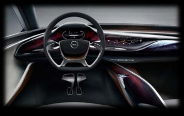
Inside, the cockpit continues the aesthetic theme of the exterior, with flowing surfaces and sweeping contours. The instrument panel features a sculpted dashboard that sweeps from door to door, and is used as a single projection surface. A total of 18 LED projectors create a continuous, adaptable multi-functional display, combining vehicle and infotainment information as well as customizable decorative elements.
