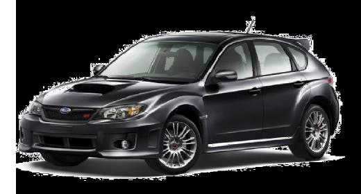
The Subaru Impreza WRX STI has become a highly optimized engine performance. Special chassis adjustment. Aluminum front lower Larms reduce unsprung weight of the vehicle. Key changes include a chassis tuning ride height lowered and new rings pillow ball front and rear cradle bushings are stiff to support the double wishbone suspension – is to increase the camber and stiffness of the foot.
