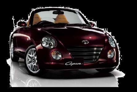
All variant Copen use 660cc turbocharged engine powered 64 hp at 6.000rpm and torque of 110Nm at 3.200Nm. Copen only has a length of 3.4 meters. Transmission can be selected, ie four-speed automatic and five-speed manual.
