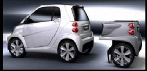
The pack can also integrate a combustion engine or range extender, packed with batteries or powered by a fuel cell, which increases the vehicle's range. In this case the docked third axle drives the rotating second axle and thus recharges the on-board battery of the city car.
