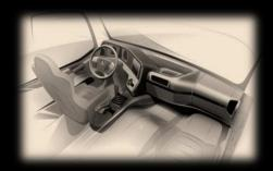
As supplements to the compact 2.3 m cabs in L, M or S versions, the new Arocs can also be fitted with spacious 2.5 m variants with a level cab floor.
