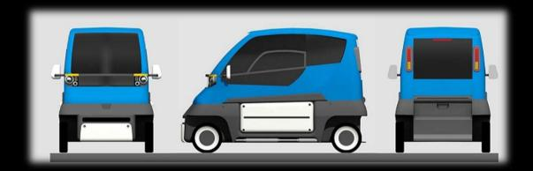
The vehicle has a unique suspension system designed by Korres Engineering that gives the vehicle a balanced ride. It can also adjust the riding height so that the back can lower to the ground (or to sidewalk level) which turns the vehicle's floor into a ramp.
