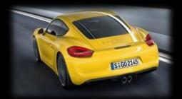
The lightweight body has a aluminum and steel mixed material design, and combined with other weight savings, allowed for a total mass reduction of 30 kg.
