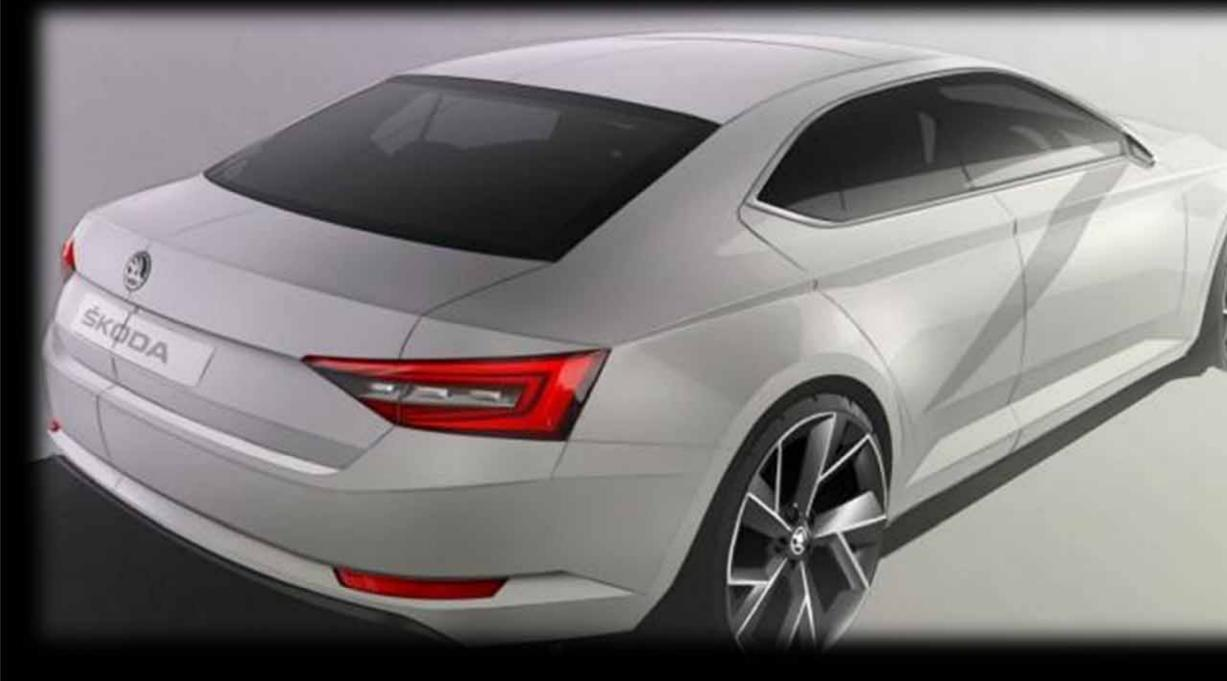
The dynamic stance is enhanced by the large wheels and the gently rearward-sloping roof line. From the sketch it is cleat that the model is the production version of the VisionC: most of the features are maintained, including the distinctive, clean treatment of the back doors with the hidden handles.
