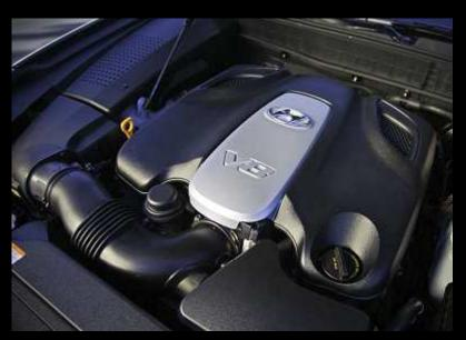
The 2011 Hyundai Equus will be competing with the best of luxury cars worldwide including the BMW 7 Series, Mercedes-Benz S-Class, Audi A8 and Lexus LS460. Under the hood of the Hyundai Equus is a 4.6-liter V8 capable of turning out 385 horsepower. There is also a rumor that Hyundai will be replacing the 4.6-liter V8 in the Equus with a more capable 5.0-liter V8.
