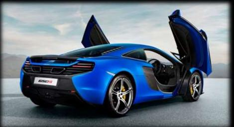
Unique side intakes behind the dihedral doors feed large, efficiently packaged, radiators which help provide the cooling requirements of the mid-mounted, compact engine. A new design five-spoke lightweight forged '650S' alloy wheel is unique to the model, and are fitted with specific Pirelli P Zero Corsa tires.
