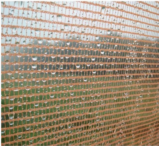
atmospheric water vapor from either rain, fog, or dew, condenses against the cold surface of the mesh
