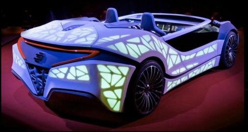
For example, it a pedestrian approaches from the right, a lighting sequence is triggered to alert the driver. Drivers' preferences as well as appointments in their diary are also taken into account in the integrated navigation system. For example, if an appointment is cancelled, the car will automatically indicate the route to the next appointment in the diary. The system also supports autonomous driving modes.
