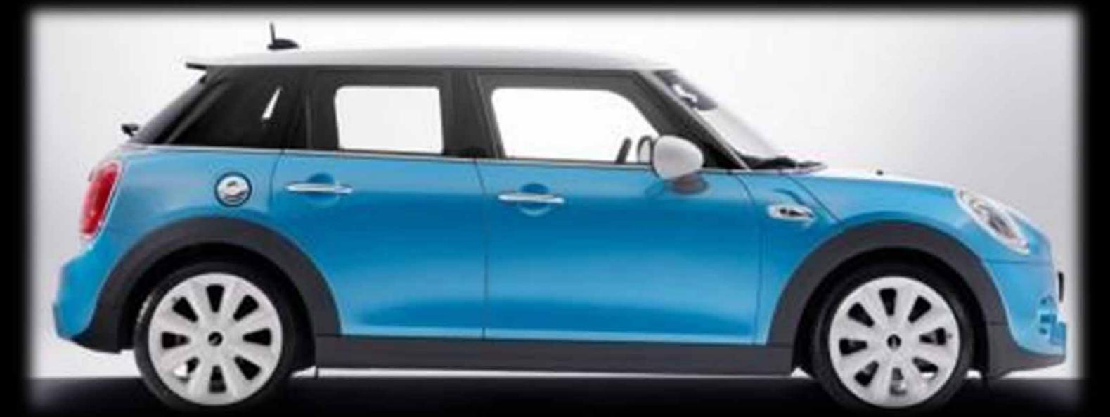
Compared to the 3 door hatchback, the new model features a wheelbase expanded by 72 millimetres and a body lengthened by 161 millimeters and a height increased by 11 mm, which result into greater interior space.
