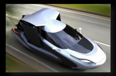
Terrafugia has presented the new design of the TF-X, the four-seat, vertical takeoff and landing (VTOL) hybrid electric aircraft, styled by designer Vedran Martinek.
