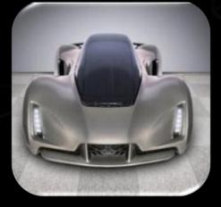
The prototype has a total weight of approx. 1,400 pounds, and is powered by a 700-horsepower bi-fuel engine that can use either compressed natural gas or gasoline. It enables a 0-60 time of about two seconds. In addition to dramatically reducing materials and energy use, the weight of the Node-enabled chassis is up to 90% lighter than traditional cars, despite being much stronger and more durable.
