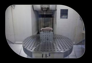
High-speed milling is a technological innovation that reduces the development time of vehicles considerably. Design models can be produced in various scales in a relatively short space of time, allowing the proportions and design elements to have their full impact.
