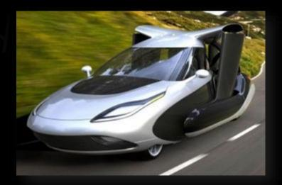
The TF-X is the evolution of the company's Transition aircraft, presented in 2013. Compared to it, it introduces two electric pods for vertical landing and showcases a more streamlined, integrated design.
