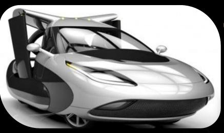
Based on the new OML, Terrafugia also developed a one-tenth scale wind tunnel test model, which is currently on display at EAA's Air Venture in Oshkosh, WI. The wind tunnel test model will be used to measure drag, lift and thrust forces while simulating hovering flight, transitioning to forward flight and full forward flight.
