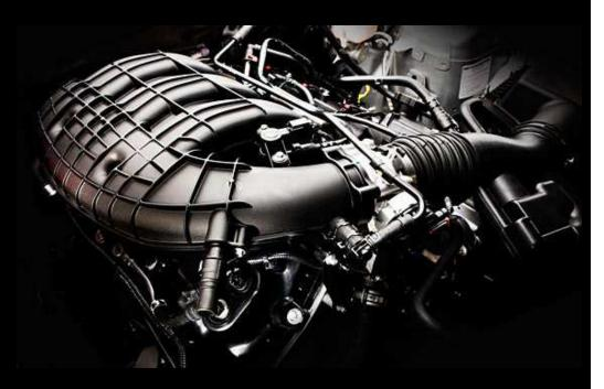
It all starts with the innovative Twin Independent Variable Cam Timing (TiVCT) technology that efficiently delivers power to this pony. The all-new 3.7-liter V6 turns out 305 horsepower with 280 lb.-ft. of torque using four valves per cylinder and TiVCT. And when all this power is projected to get 30 mpg hwy,\* you know the 2011 Mustang V6 is destined to change the game.
