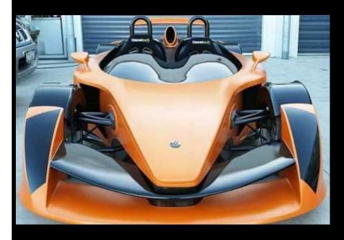
The Hulme Can Am is an ultra high-performance, midengined roadster created for both road and track use. Entirely designed and hand-built by the Hulme Supercars technology team in New Zealand, the road-legal car features an ultra-lightweight carbon composite tub and bodywork and weighs in at less than 1000kg. Powered by a Chevrolet LS7 V8 developing 600bhp, the Can Am measures 4712mm in length, 1958mm wide, 1095mm high, and rides on a 2830mm-long wheelbase.
