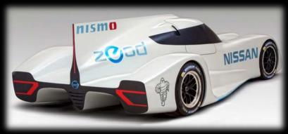
The ZEOD is expected to race alternately using gasoline and electric power.
