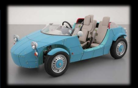
The interior features three seats arranged in a 1+2 triangular configuration
