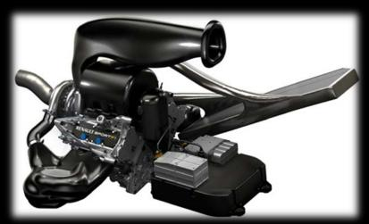
Formula 1 moves from the naturally aspirated 2.4-litre V8 engine configuration it currently uses to a more environmentally acceptable 1.6-litre turbo charged V6 formula next year. Renault has become the latest manufacturer to unveil its engine for next year and has named it the Energy F1-2014.
