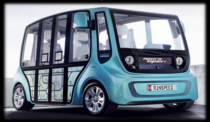
The main feature of the vehicle is the height of almost 2.2 meters, which allows the installation of space-saving upright seats equipped with a custom- developed safety belt system from TRW.
