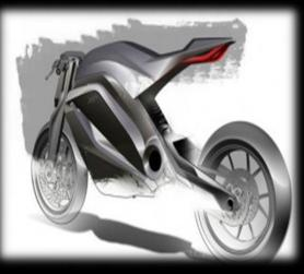
The Motorrad Concept is powered by a Ducatiderived 850cc, L-Twin cylinder, 4 valve per cylinder, Desmodromic 2-cylinder engine coupled with a double clutch gearbox.
