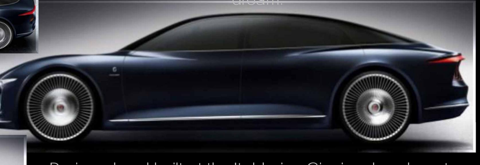
Designed and built at the Italdesign Giugiaro headquarters in Moncalieri, the GEA concept is based on the "Piloted Driving" technology and is characterized by generous proportions – it is 5.37 meters long, 1.98 m wide and 1.46 meters high, while the wheelbase is 3.33 meters long. The powertrain features four electric motors fitted on the differentials, developing a total of 570 k, enabling a top
