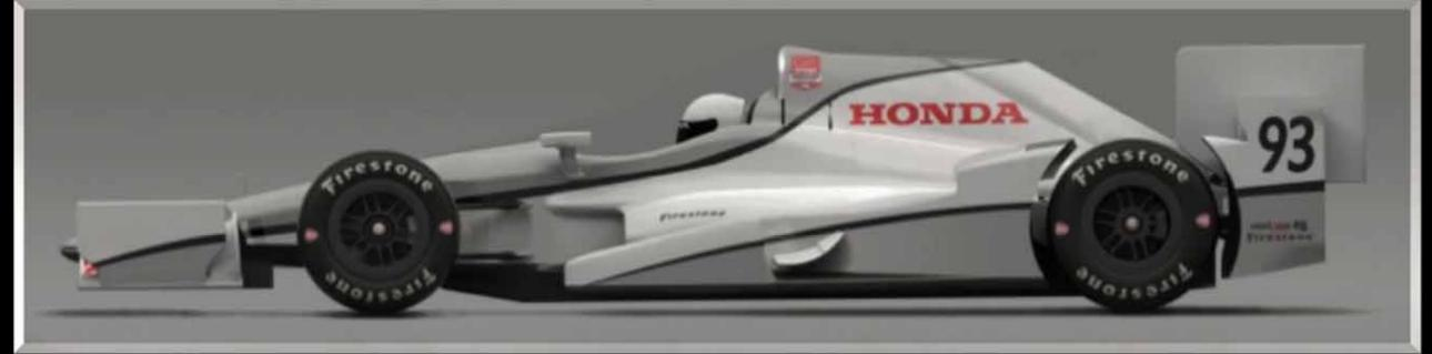
The extreme-looking kit, produced by Honda Performance Development, Honda's racing arm in North America, consists of 200 carbon-fiber pieces that can be fitted to the existing Honda-powered Dallara Indy car chassis, allowing teams to customize the configuration depending on the specific circuits, driving styles and track conditions.
