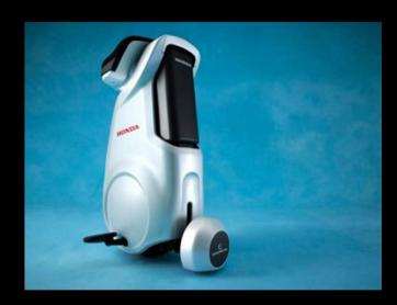
The main features of the concept are Honda's proprietary balance control technology and the Omni -directional driving wheel system (Honda Omni Traction Drive System).
