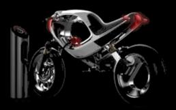
The engine is visually replaced by a symbolic void, while the electric motor is positioned in the hubless rear wheel.
