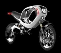
The entire bottom chassis is dedicated to storing battery cells. This location lowers the bikes center of gravity, creating an extremely stable ride. Because the motorcycle's speed is controlled directly by the power to the electric motor, virtually all other major mechanical components of a traditional motorcycle are no longer required".
