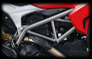
Steel trellis frame, a diecast/ techo-polymer mix subframe and diecast single-sided swingarm. The fork is a nonadjustable 43mm Kayaba unit, while the single Sachs rear shock is adjustable for preload and rebound damping. Dry weight is a claimed 181kg, only 6kg heavier than the standard Hypermotard.
