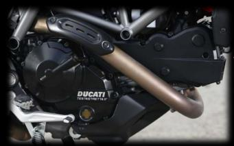
It's 110bhp, 65.8ftlb, watercooled, 821cc, 4v, Testastretta 11° V-twin motor as the standard Hypermotard and SP. A major (valve check) service is recommended at 18,000 miles.
