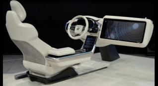
Concept 26 features a tablet interface in the center console, a foldable tray table and a 25-inch flat-screen monitor that flips up from the passenger side dashboard, and offers three interior modes: Drive, Create and Relax.
