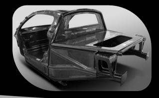
iStream® Carbon can cater with annual production volumes between 1,000 and 350,000 units per year at a cycle time of 100 seconds and can reduce capital investment by up to 80% reducing manufacturing energy by up to 60% whilst offering new levels of rigidity, corrosion resistance, safety, durability and low cost light weighting.
