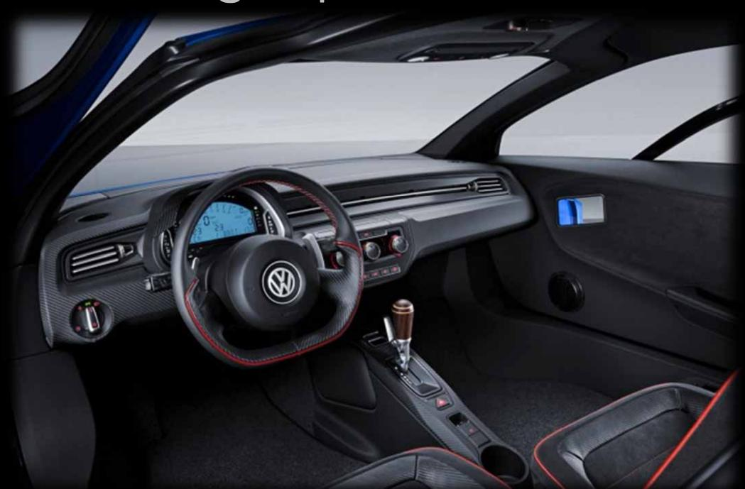
The door windows are made of polycarbonate. The upper part of the windows is firmly attached to the exterior door skin due to the specifications of lightweight design, while a segment of the lower area of the side windows can be opened. The windscreen of both models is manufactured from a special type of thin glass. The XL Sport's steering wheel has decorative red stitching and has been equipped with aluminium shift paddles to facilitate ultra quick gear shifts.
