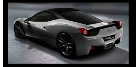
The Ferrari 458 Italia's performance: 0-100 km/h acceleration in under 3.4 seconds and a maximum speed in excess of 325 km/h. For the new chassis, once more in aluminum, Maranello's engineers incorporated various types of advanced alloys along with aerospace industry-derived manufacturing and bonding techniques.
