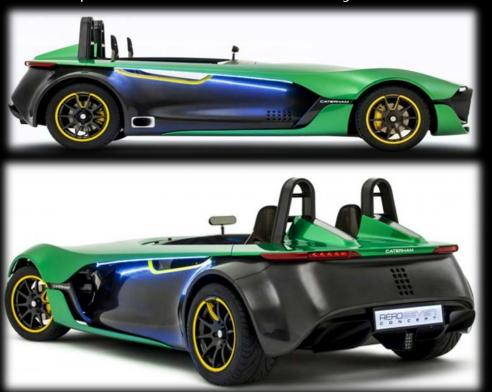
The exterior design is based on the combination of different layers: the top, body-painted half stretches above the underlying body panels in exposed carbonfiber, while at the front a lower wing visually balances matches the shapes of the hood. The AeroSeven is equipped with a Euro 6 compliant Ford Duratecbased engine delivering 240ps (237bh, which allows the sportscar to sprint from zero to 100kph in under 4 seconds. Power is transferred to the rear wheels via
